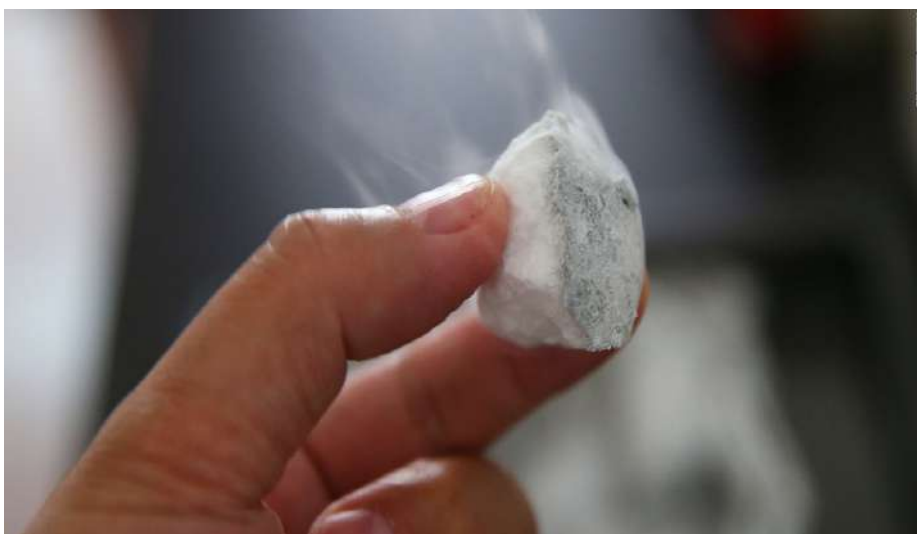
A scientist holds marine natural gas hydrate trapped in icelike crystals, extracted from the seabed of the Shenhu Area of the northern South China Sea. Similar marine natural gas hydrates have been extracted from Japan.
