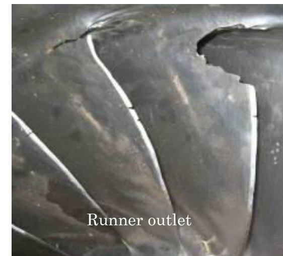
4 MW*3 Francis runner at Jhimruk Hydroelectric Center, Nepal Ref: O.G. Dahlhaug, 2004
