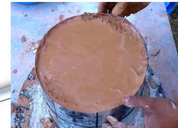
Plaster mold for runner
