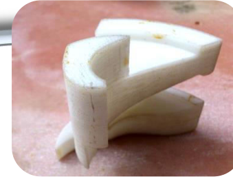
Plastic section of a runner sector
