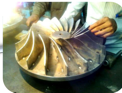
Assembly of the runner blades
